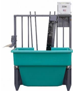
Figure 1. The SmartFeed system integrates feed bin, load cells, and RFID reader to log cattle feed intake quantity each time an animal visits the feed bunk.
