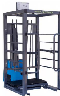
Figure 2. SmartScale is a wireless scale system that integrates load cells and RFID to log partial body weight and behavior each time an animal visits the waterer.
